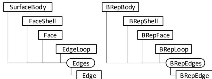
There are several ways to access edges through the API. From a body or shell object, you can get an Edges/BRepEdges collection that contains all of the edges in the body. From a Face/BRepFace object you can get the edges associated with the face; either all at once or loop by loop, using the EdgeLoop/BrepLoop object.
