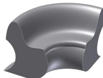
The important thing to understand is that a face represents a surface but does not define anything about the shape of that surface. The same is true of edges; they represent a curve but do not define the shape of the curve. The primary purpose of the topology objects is to define how the various geometries are connected. To fully understand the shape of the model, you need to look at the geometry associated with the topology object.
