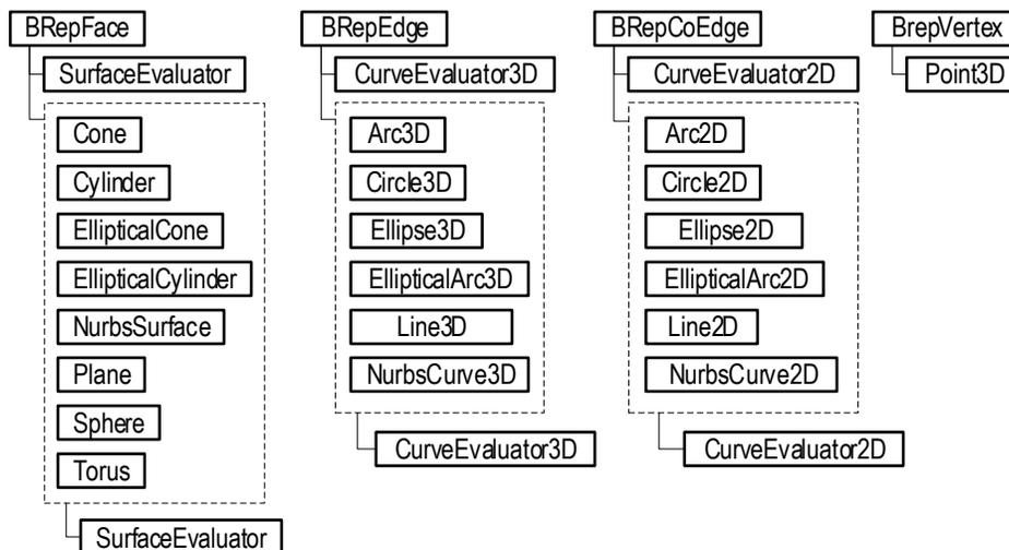
In Inventor, in addition to the Geometry property, the Face object also supports the SurfaceType property, and the Edge and EdgeUse objects support the GeometryType property. These properties return an enum value that specifies the type of geometry represented by the B-Rep entity. It's an easy way to determine what type of object the geometry property will return. In Fusion 360 you need to get the geometry and then check the type of object returned.
