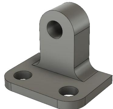
1. As with all parts, we begin by creating a sketch. In this case, the base XY construction plane has been chosen as the sketch plane, a rectangle of the correct size has been drawn and used to create an extrusion.
