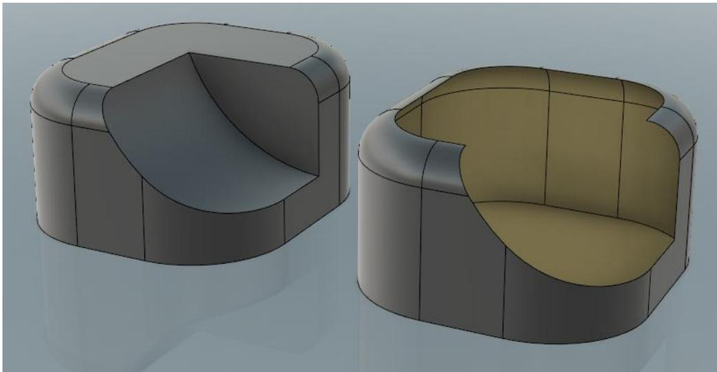
There are two concepts you need to understand to be able to work with a B-Rep model; *topology* and *geometry*, which are described in the sections below along with the API functionality that lets you access this information. An important point to understand is that the functionality described is providing read-only access to the model. It does not provide any editing capability. Editing of an Inventor or Fusion 360 model is always done through features.
