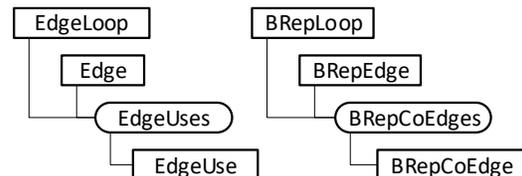
The other big difference between EdgeUse/BRepCoEdge objects and edges is that the EdgeUse/BRepCoEdge object is not a 3D object. (All other B-Rep objects are 3D objects.) EdgeUse/BRepCoEdge objects are defined in the 2D parametric space of a face. The concept
