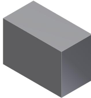
The three models shown below are examples of other models made up of 6 faces and 12 edges. All these models have the same topology but obviously have radically different geometry.
